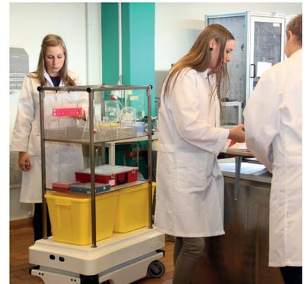
MiR100 can be outfitted with various modular solutions depending on the type of goods or materials needed to transport.
